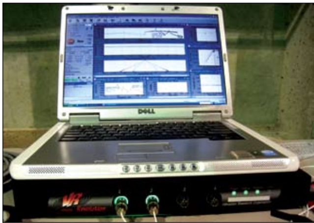
Figure 11. VR9500 Revolution controller runs multiple specimens to destruction using NAVMAT profile.
