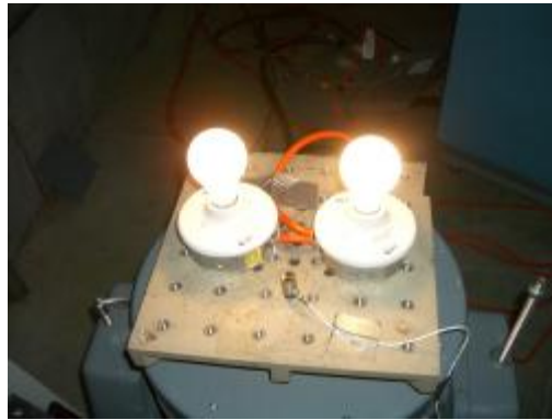
Figure 11. Setup for vibration testing of light bulbs with kurtosis.
