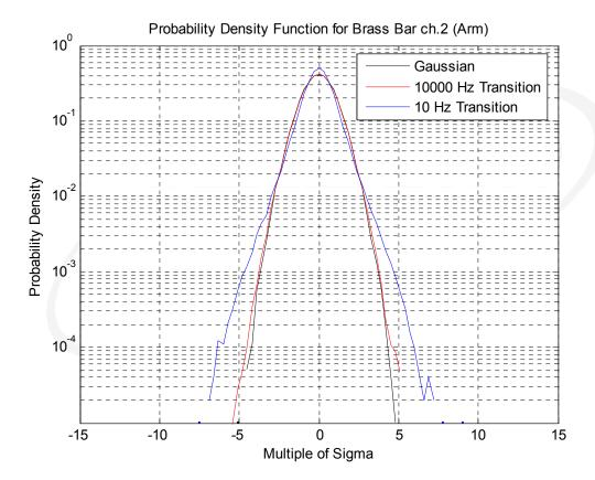
PDF for the Brass Bar (Arm) Data for tests with Gaussian distribution, Kurtosis = 5 (Transition 10,000 Hz) and Kurtosis = 5 (Transition 10 Hz).
