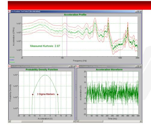
Spectrum defined by field measured data Traditional random test with 3 sigma clipping
