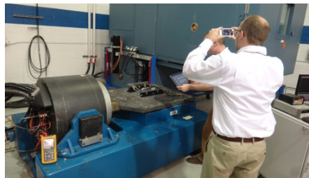
Figure 12: FORD Boss Fuel-Rail System on a shaker
