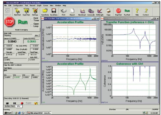
Figure 19. Closing loop around challenge filter with VR 8500 using 800 lines of resolution.
