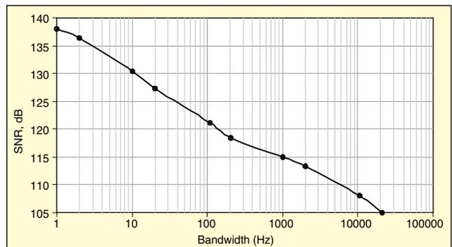
Figure 8. Dynamic range of the VR 8500 controller at various bandwidths.
