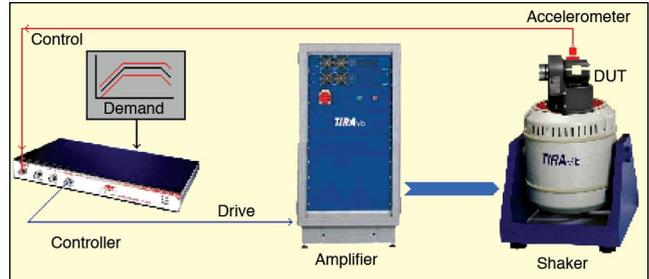
Figure 1. Vibration controller generates drive signal that causes measured control acceleration to closely match prescribed demand.
