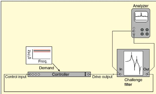
Figure 18. Testing dynamic range by closing loop around simulation filter.
