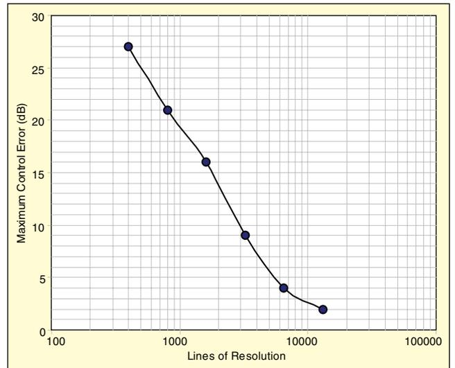
Figure 23. Maximum loop-error versus random control resolution shows at least 8,000 lines of resolution required to hold challenge filter in control within  $\pm 3$  dB over the NAVMAT band.
