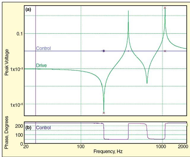
Figure 25. VR 8500 control and drive signals during a swept-sine test.
