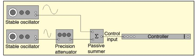
Figure 3. Testing dynamic range of control input using the two-tone method.
