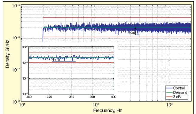
Figure 22. A 13,000-line control signal spectrum-analyzed by an external analyzer.
