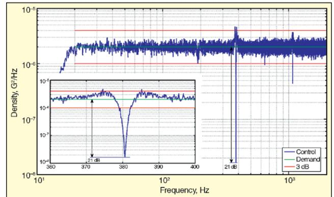
Figure 20. An 800-line control signal spectrum-analyzed by an external analyzer with more resolution.
