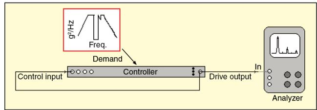
Figure 15. Testing both drive and control dynamic range using a severe demand.
