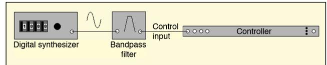
Figure 5. Testing the dynamic range of a control input using the IEEE effective-bits method.
