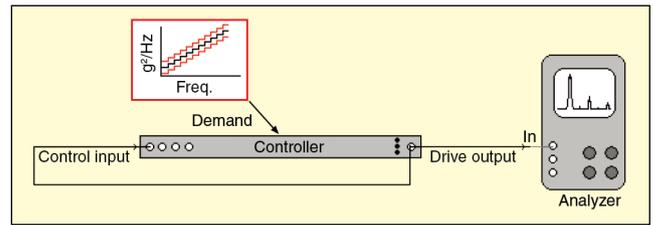
Figure 13. Narrow-band random loop-back test setup.
