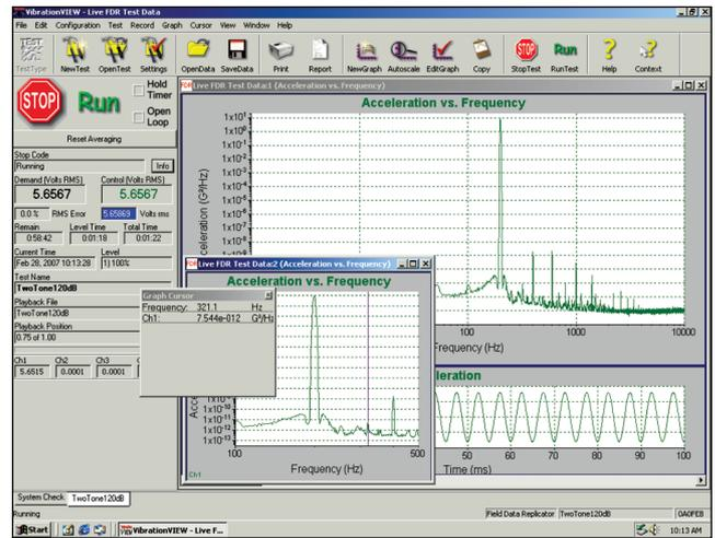
Figure 4. Two-tone test of VR 8500 controller indicates 120 dB between full-scale and small tone.
