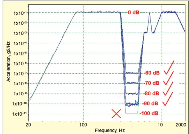
Figure 16. VR 8500 performing Chinese JJG 529-88 challenge test at 60, 70, 80, 90 and 100 dB.
