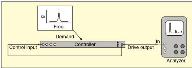
Figure 9. Testing dynamic range of drive output.
