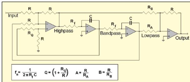
Simplified schematic of a filter section; challenge filter is comprised of two differently tuned sections in series.
