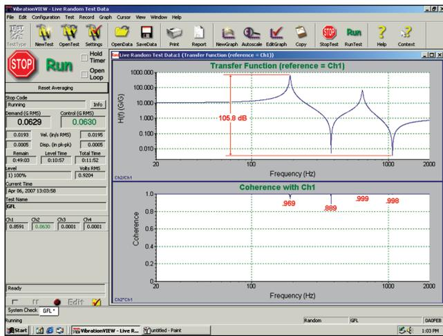
Figure 24. A 13,000-line transfer function of challenge filter shows more than 105 dB of dynamic range; corresponding coherence function indicates an extremely 'clean' measurement.
