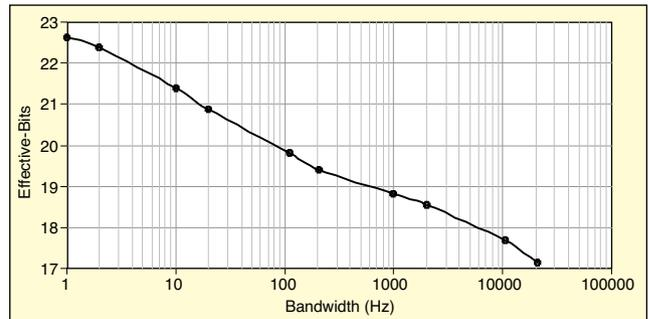
Figure 7. Measured effective bits of the VR 8500 control input channel at various bandwidths.
