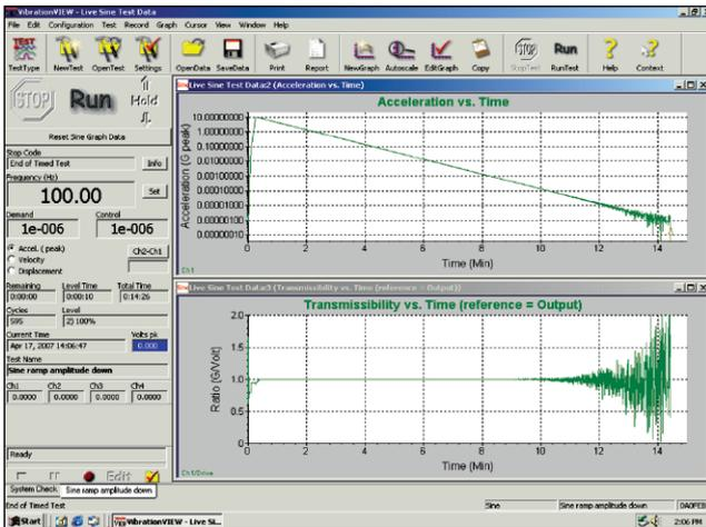
Figure 12. Ramped-sine test of VR 8500 controller indicates about 120 dB input/output dynamic range.
