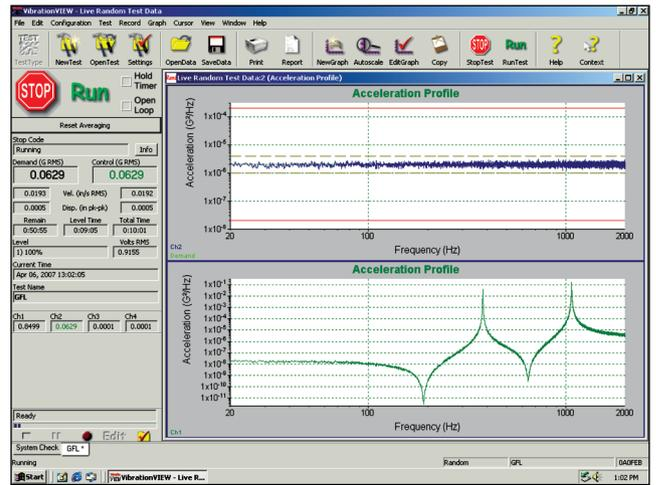
Figure 21. Closing loop around challenge filter with 13,000 lines of resolution.
