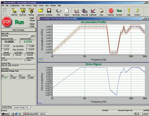
Figure 17. Details of JIG 529-88 operation at 90 dB showing control with limits and drive signal.
