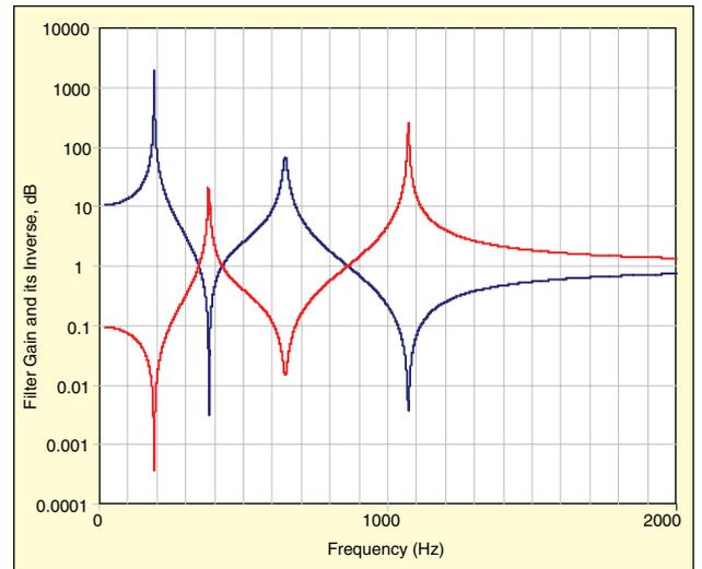
loss at the lowest notch must be known in advance. For the sample case here, the filter transfer function has a 50-dB loss at the lowest notch, so the demand level must be at least 50 dB lower than the maximum achievable output voltage. For a controller with a 10 V maximum, we choose a demand level of  $0.01 V_{peak}$ , or 60 dB below the maximum.
