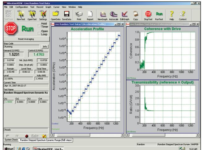
Figure 14. Random test indicates 100 dB of clean dynamic range for VR 8500.
