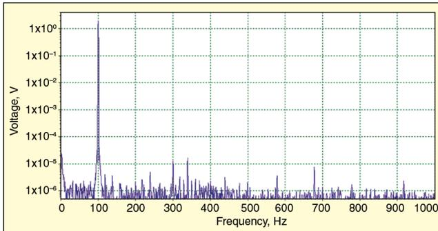
Figure 10. Single-tone test of VR 8500 drive output shows more than 100 dB dynamic range.
