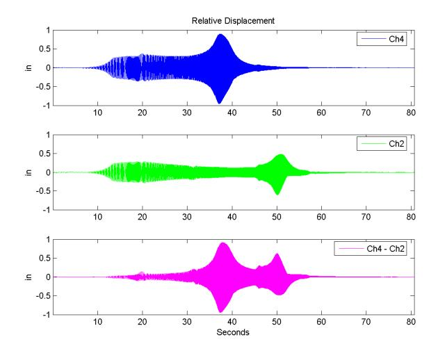
The graph above shows the displacement vs time of channel 4, channel 2 and the relative displacement between the two. It may not be clear from the graph above, but the maximum and minimum values do not occur at the same time. The maximum value of 0.91 inches occurs at 37.9 seconds and the minimum value of -0.94 inches occurs at 37.5 seconds.
