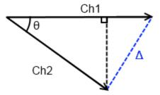
The relative displacement between Ch 1 and Ch 2, labeled  $\Delta$ , can be calculated with the following equation.
