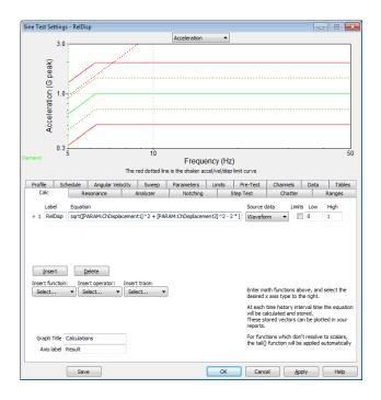
NOTE: the [PARAM: ChDisplacement1] is divided by 2. That is because the PARAM value is peak to peak. The equation requires the amplitude.
