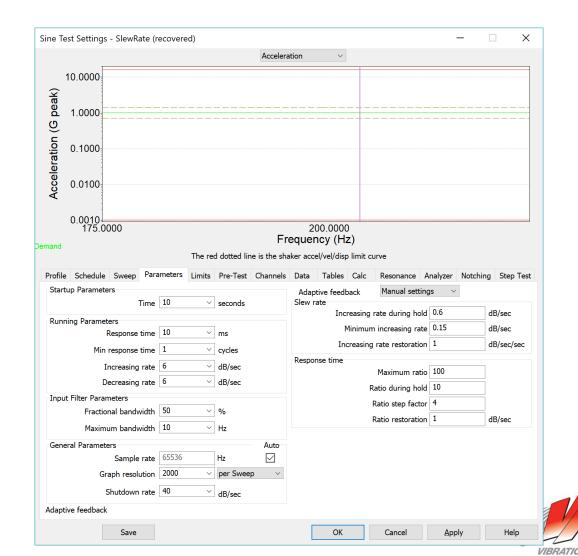
These settings allow tighter control during the test but still limit problems in a resonance
