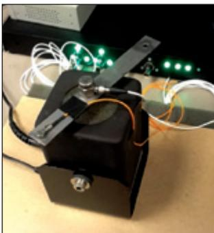
Figure 3. Tear-drop accelerometer attached to beam's "short arm."
