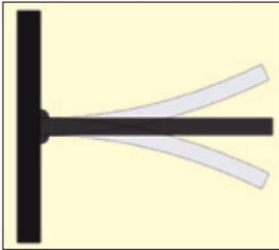
Figure 1. Resonating cantilevered beam - profile.
