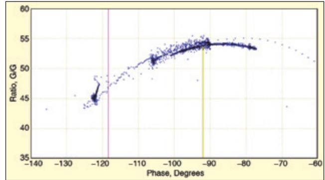
Figure 10: Screenshot of VibrationVIEW software showing use of advanced user-defined SRTD phase-tracking control to obtain higher peak transmissibility; peak transmissibility occurs around  $-90^\circ$  and not the predicted  $-105^\circ$ .
