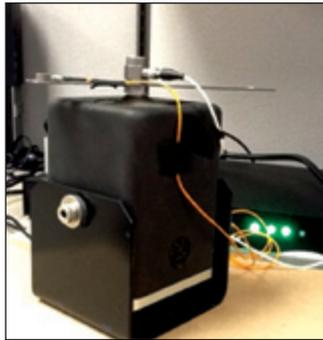
Figure 7: Thin metal beam attached to shaker.
