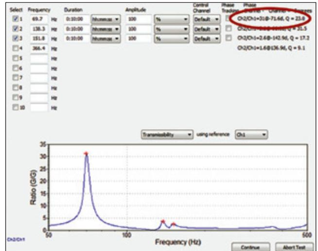
Figure 4. Resonance table for metal beam (long arm), showing fundamental resonance at 69.7 Hz with peak transmissibility of 31 G/G and a phase of -71.6°.
