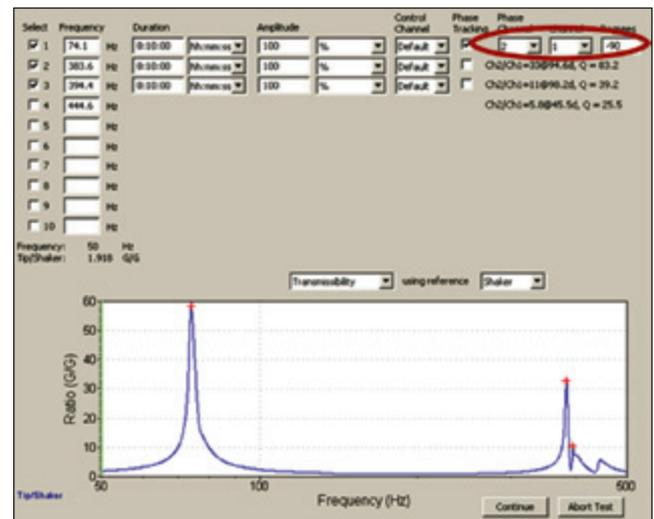
Figure 5. Phase-tracking setting selected for lawnmower blade test; phase is automatically set to 90°.
