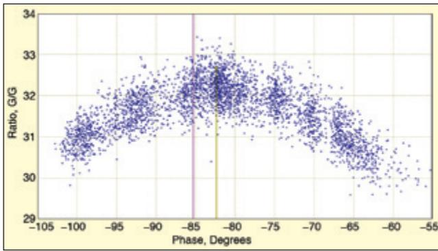
Figure 6. Transmissibility metal beam tip (long end of beam) to shaker head vs. phase of resonance. Standard SRTD predicts a phase of  $-71.6^\circ$  (peak transmissibility of 31 G/G) and the phase tracking sets phase to default of  $-90^\circ$ ; meanwhile, a new feature, advanced user-defined SRTD phase-tracking control, allows adjusting phase to  $-82.5^\circ$  to obtain the true peak transmissibility (32.4 G/G).
