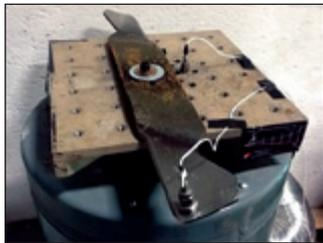
Figure 8: Lawnmower blade attached to large shaker.
