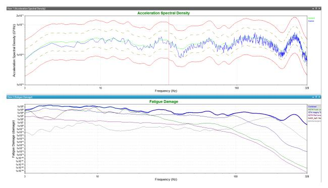
The Random PSD generated is the damage equivalent to the lifetime of the product based on the imported files, *m* and Q values, Target Life, Test Duration, and kurtosis. This is valuable information in every phase of testing from initial product development to re-creating field failures in a lab environment.
