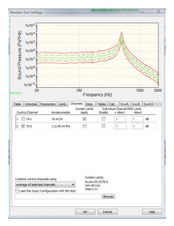
**Step 6.** The new test profile is saved and now may be used to run the vibration test with acoustic control on channel 2.
