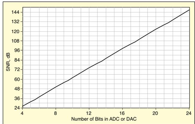
Figure 6. Relationship between effective bits and dynamic range or SNR.
